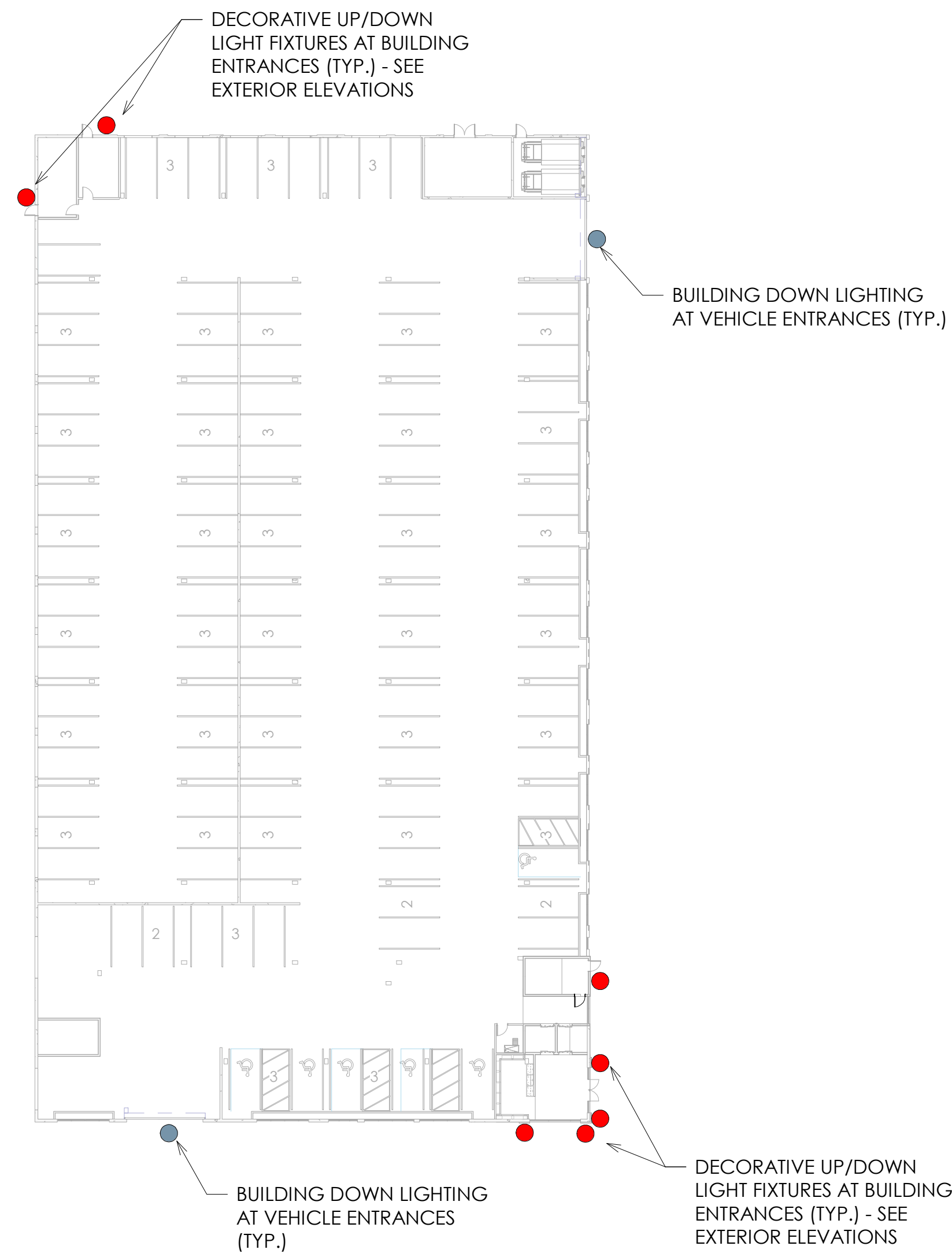
2 A101 MAIN LEVEL EXTERIOR LIGHTING PLAN 1/32" = 1'-0"
