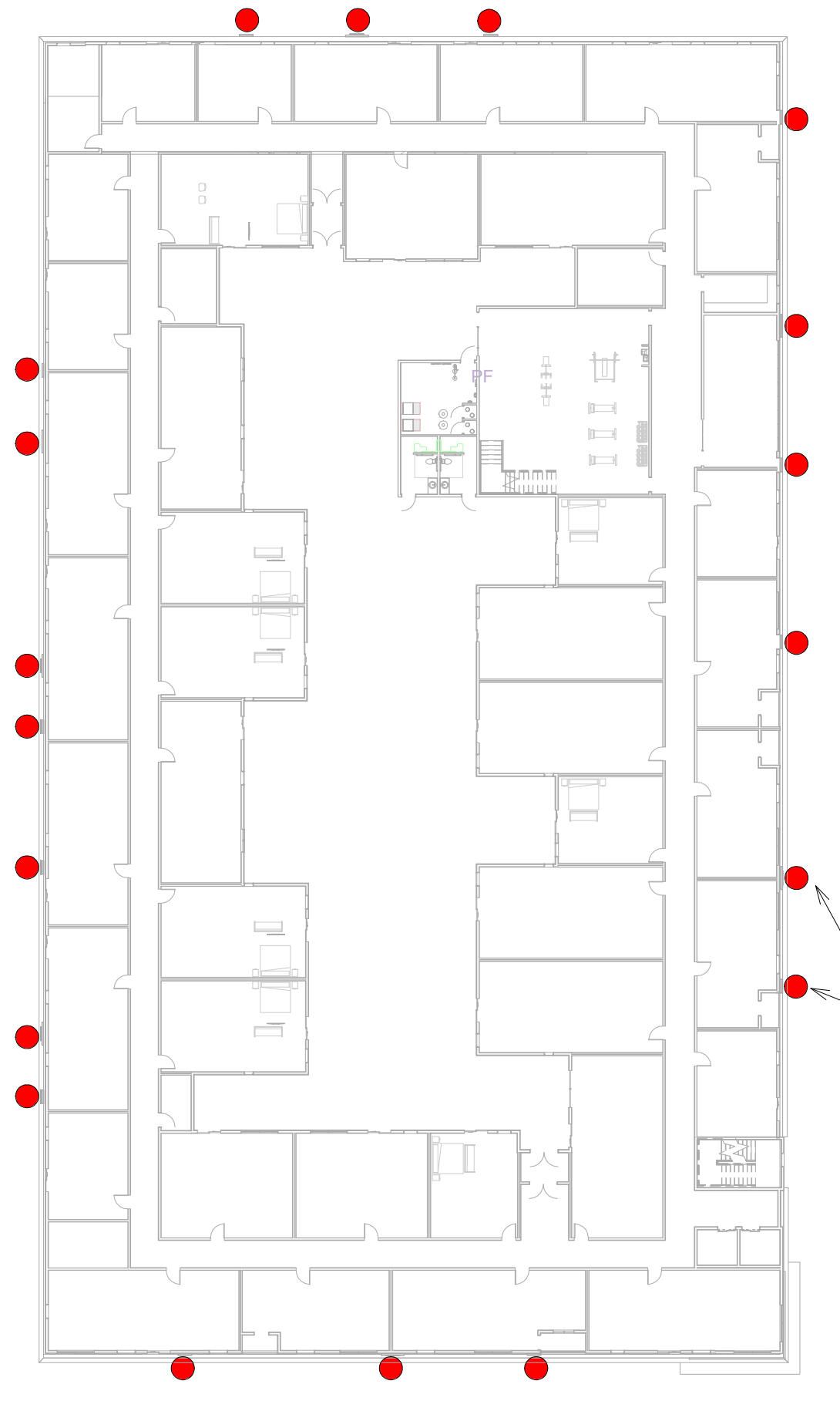
2 THIRD LEVEL EXTERIOR LIGHTING PLAN 1/32" = 1'-0"
